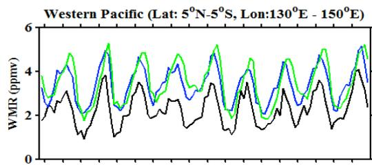
Fig. 5 MLS measured water vapor mixing ratio at 100hPa (blue line) and 82 hPa (green line). The water vapor saturation mixing ratios estimated for CPT temperatures are represented by black line.
