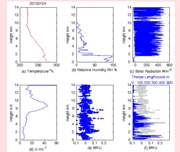
Fig 3. (a) temperature, K (b) relative humidity, % (c) solar radiation,  $W m^{-2}$  (d) wind speed,  $m s^{-1}$  (e) MVU (f) calculated Thorpe length scale, m (blue) over-plotted on MVU (grey) at 1100 on 24/01/2013.
