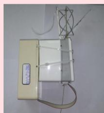
Fig 2. Instrumentation setup: PANDORA box containing magnetometer sensor and solar radiation sensor (left) attached to RS92 radiosonde (right)
