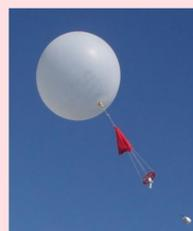
Fig 1. RS92 radiosonde flown beneath a 200g balloon (University of Reading)
